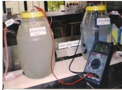
Fig.1. MFC setup in laboratory
